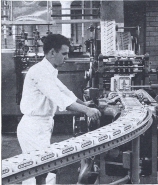
MARGARINE PRODUCTION . . . VOTATOR Margarine Processing Apparatus produces margarine of uniform texture, consistency, and weight. The process is continuous, completely enclosed, automatic.
